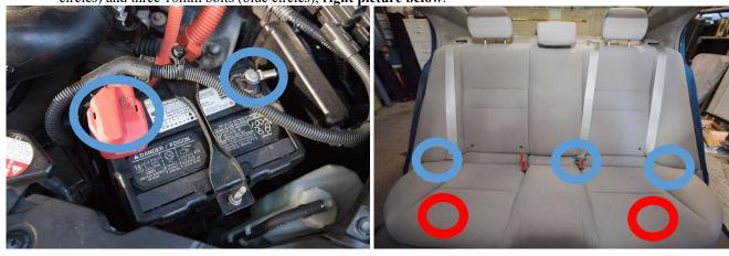
3. Remove the IMA switch cover plate, two T30 bolts (blue circles), left picture below.
